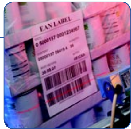
Barcode checking before and after application
