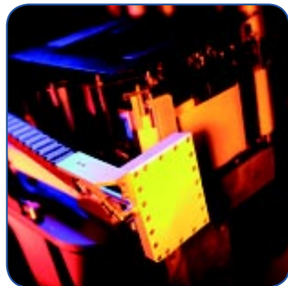
Tamp application tool for top labelling
