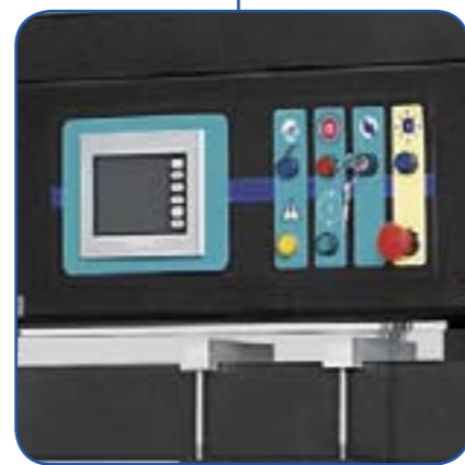
The linear, bi-axial and traversing movements are individually controlled from the exterior touch panel
