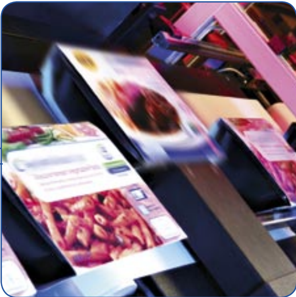
Incorrectly packaged product is removed into an intelligent reject bin
