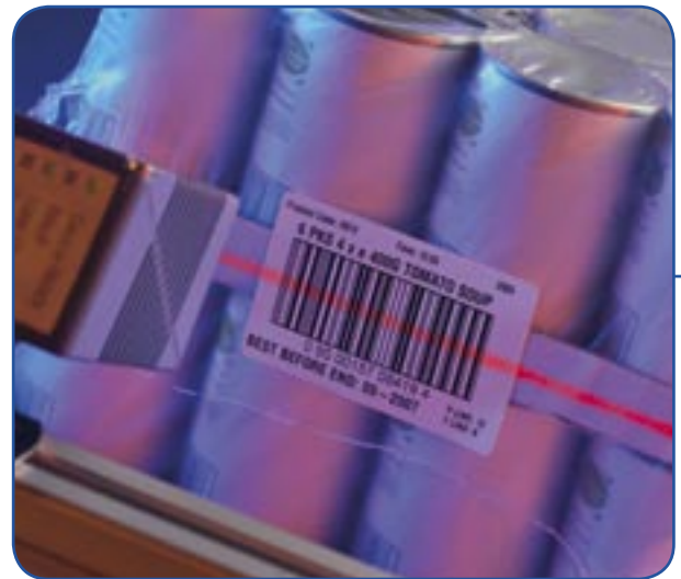
Verification after apply guarantees barcode quality and label positioning
